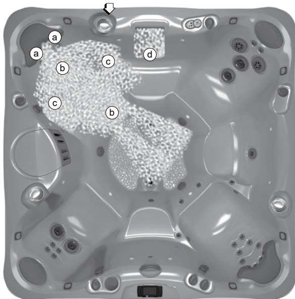
JET PUMP 2 – JET SYSTEM 1
