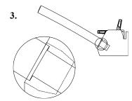
Insert wire fully into Terminal Block
