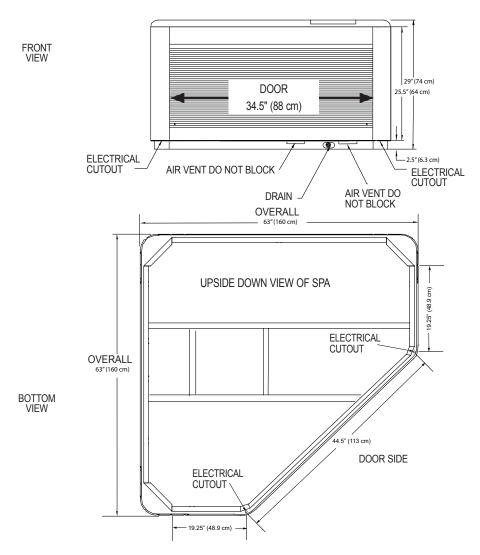
**NOTE: WATKINS WELLNESS** recommends that the **AVENTINE** be installed on a minimum 4" (10 cm) thick reinforced concrete pad or structurally sound deck able to support the "dead weight" found in the spa specification chart.
