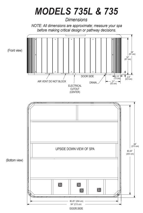
**NOTE: WATKINS WELLNESS** recommends that the spa be installed on a minimum 4" (10.2 cm) thick reinforced concrete pad or structurally sound deck able to support the "dead weight" found in the spa specification chart.
