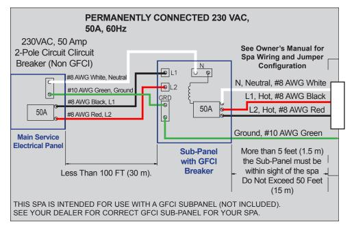
**INSTALLATION NOTE:** After the spa has been installed, your electrician can connect the conduit from the subpanel to the spa's control box and then complete the wiring connections in the control box. **NOTE:** Complete step-by-step Installation and Wiring Instructions for all models are included in the Owner's Manual.
