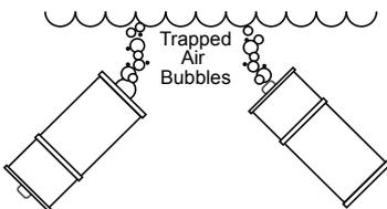
Submerge assembled filter in spa and tilt each end upward to remove trapped air bubbles from inside each filter cavity.
