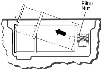
Loosen filter nut to provide clearance, then remove filter assembly.
