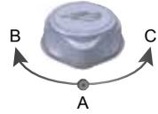
**Note:** The massage selector is designed to operate in positions A (Combo), B, and C for optimum performance. It is considered normal for sound levels within the valve to vary between positions due to the large amounts of water flowing through it. For optimum filtration benefits, leave the valve in position A when spa is covered. Select position B or C for maximum jet performance during spa use.
