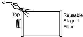
Rinse debris from all filter pleats using a garden hose and high-pressure nozzle. Start at top and work downward to face. Repeat process until all filter pleats are clean.
