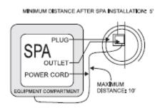
This is a picture of what your 115v spa will look like once you have the proper electrical outlet installed. The spa dealer is **not** licensed to do electrical and does **not** perform any electrical or contractor work needed or required for your hot tub.
