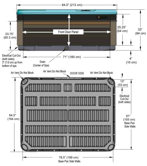
NOTE: WATKINS WELLNESS recommends that the RAVELLO be installed on a minimum 4" (10 cm) thick reinforced concrete pad or structurally sound deck able to support the "dead weight" found in the spa specification chart.
