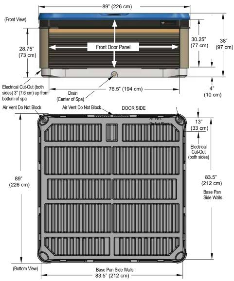
**NOTE: WATKINS WELLNESS** recommends that the **GENEVA** and **NIAGARA** be installed on a minimum 4" (10 cm) thick reinforced concrete pad or structurally sound deck able to support the "dead weight" found in the spa specification chart.
