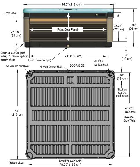
**NOTE: WATKINS WELLNESS** recommends that the **TAHITIAN** and **FLORENCE** be installed on a minimum 4" (10 cm) thick reinforced concrete pad or structurally sound deck able to support the "dead weight" found in the spa specification chart.
