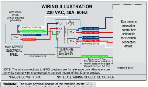
breaker will vary between manufacturers. Connecting the hot wire to the neutral terminal will cause irreversible damage to the control box.
