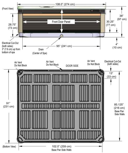
NOTE: WATKINS WELLNESS requires that the CANTABRIA be installed on a minimum 4" (10 cm) thick reinforced concrete pad or structurally sound deck able to support the "dead weight" found in the spa specification chart. WARNING: The CANTABRIA must not be shimmed in any manner.
