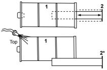
NOT use chemical cleaners or high-pressure nozzle on insert (2) or it may be damaged, come apart or allow impurities to re-enter the water, increasing the risk of contracting a waterborne illness (e.g., an infection bacteria or virus) and/or respiratory ailments.
