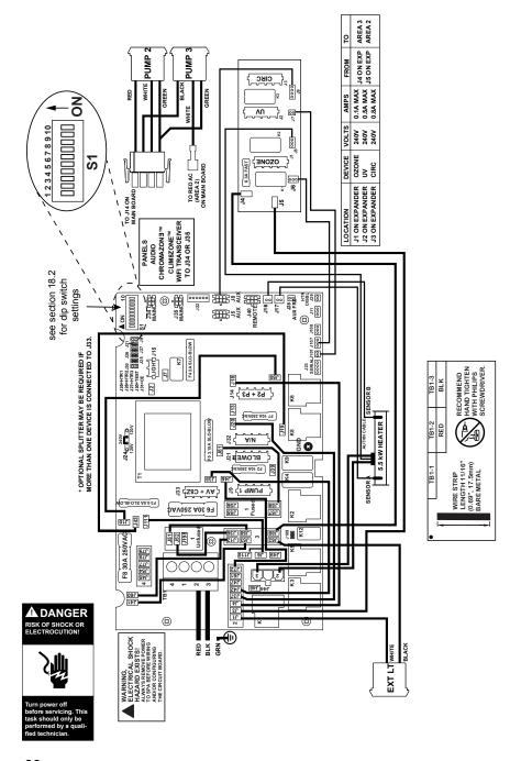
**18.2 Dip Switch Settings**The dip switches are at the S1 location on the board.
