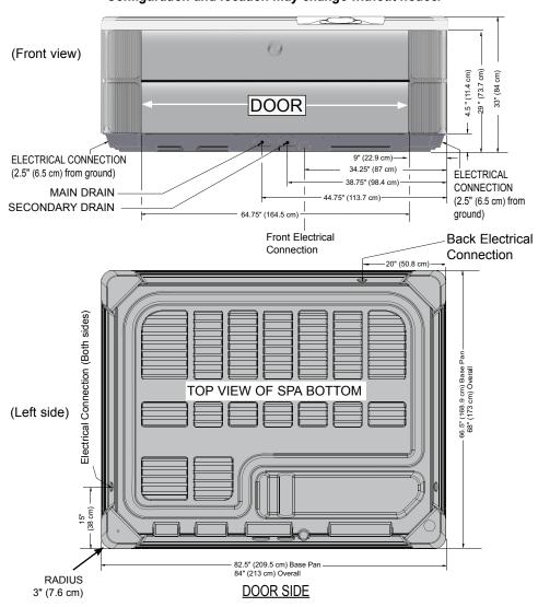
**NOTE: WATKINS WELLNESS** recommends that the **JETSETTER** be installed on a minimum 4" (10 cm) thick reinforced concrete pad or a deck that is able to withstand more than 115 lbs/ft² (555 kg/m²).
