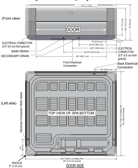
**NOTE: WATKINS WELLNESS** recommends that the **PRODIGY** be installed on a minimum 4" (10 cm) thick reinforced concrete pad or a deck that is able to withstand more than 125 lbs/ft² (595 kg/m²).
