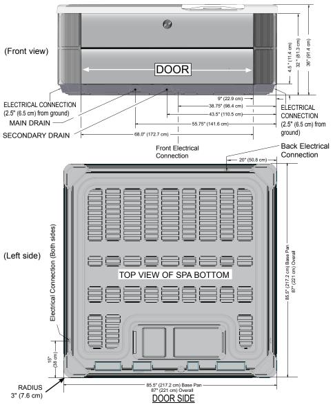
**NOTE: WATKINS WELLNESS** recommends that the **VANGUARD & ARIA** be installed on a minimum 4" (10 cm) thick reinforced concrete pad or a deck that is able to withstand more than 130 lbs/ft² (630 kg/m²) & 125 lbs/ft² (595 kg/m²).
