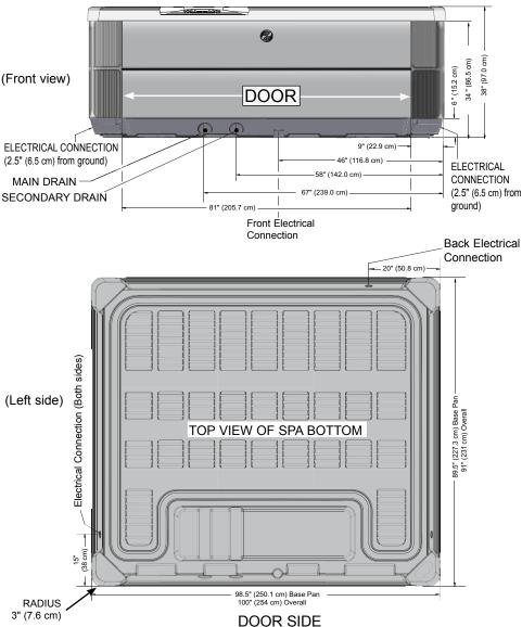
**NOTE: WATKINS WELLNESS** requires that the **GRANDEE** be installed on a minimum 4" (10 cm) thick reinforced concrete pad or a deck that is able to withstand more than 125 lbs/ft² (605 kg/m²).
