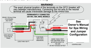
the Relay & Rhythm spa models only. Purchase the subpanel from you dealer for the converted models when converting to 230 volts.
